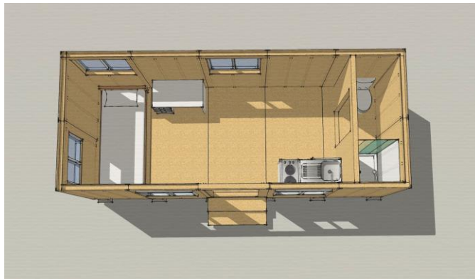
Simple illustrative drawing of an 8'x20' tiny house that meets the 2012 IRC minimum area requirements
